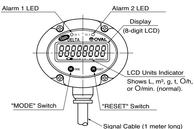
MODE/RESET is selectable with selector magnet furnished with the unit.
